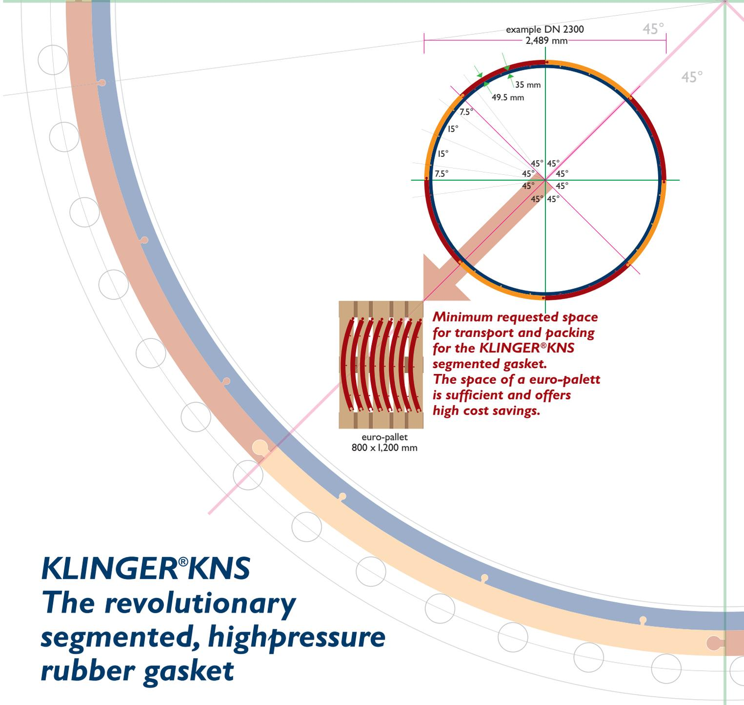
**Minimum requested space for transport and packing for the KLINGER®KNS segmented gasket. The space of a euro-pallet is sufficient and offers high cost savings.**
