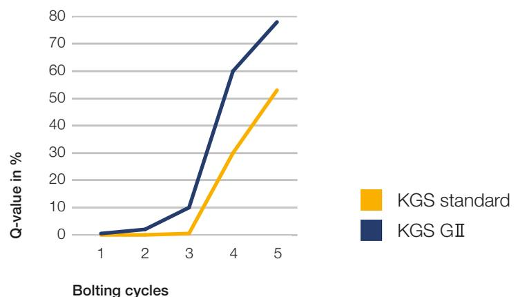
>> The quality gain after five bolting cycles can be clearly recognised in the diagram
